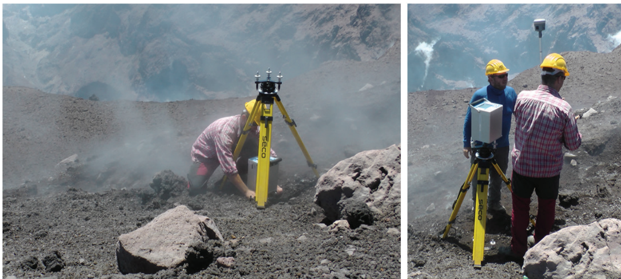
Fig. 3. In situ VGG observations on Etna (NE crater) using a relative gravimeter in tower mode.
