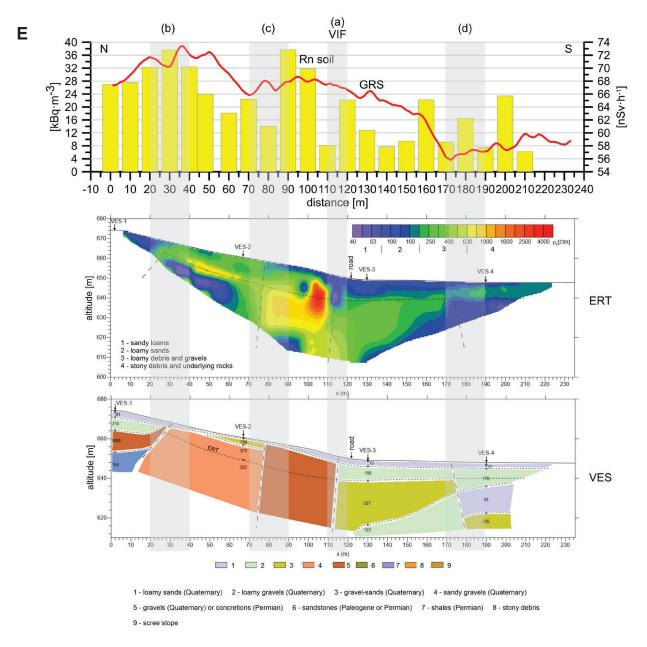
Fig. 5. (continued) Comparison of CSAMT related fault structures and shallow depth geophysical, emanometric and dowsing data. A — Kravany profile; B — Spišský Štiavnik profile; C — Vydrník profile; D, E — Spišské Bystré profiles; F — Hranovnica–Dubina profile. Geophysically detected single faults are distinguished by alphabet indications (a – VIFs.s., b, c, ...) commented in the text. Grey transparent belts mark and connect multi-method indications of the same fault-discontinuity.
