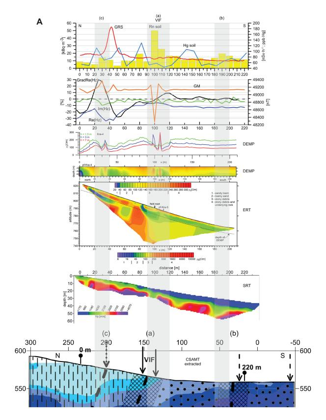
Fig. 5. Comparison of CSAMT related fault structures and shallow depth geophysical, emanometric and dowsing data. A — Kravany profile; B — Spišský Štiavnik profile; C — Vydrník profile; D, E — Spišské Bystré profiles; F — Hranovnica–Dubina profile. Geophysically detected single faults are distinguished by alphabet indications (a – VIFs.s., b, c, ...) commented in the text. Grey transparent belts mark and connect multi-method indications of the same fault-discontinuity.
