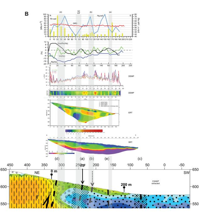
Fig. 5. (continued) Comparison of CSAMT related fault structures and shallow depth geophysical, emanometric and dowsing data. A — Kravany profile; B — Spišský Štiavnik profile; C — Vydrník profile; D, E — Spišské Bystré profiles; F — Hranovnica–Dubina profile. Geophysically detected single faults are distinguished by alphabet indications (a – VIFs.s., b, c, ...) commented in the text. Grey transparent belts mark and connect multi-method indications of the same fault-discontinuity.
