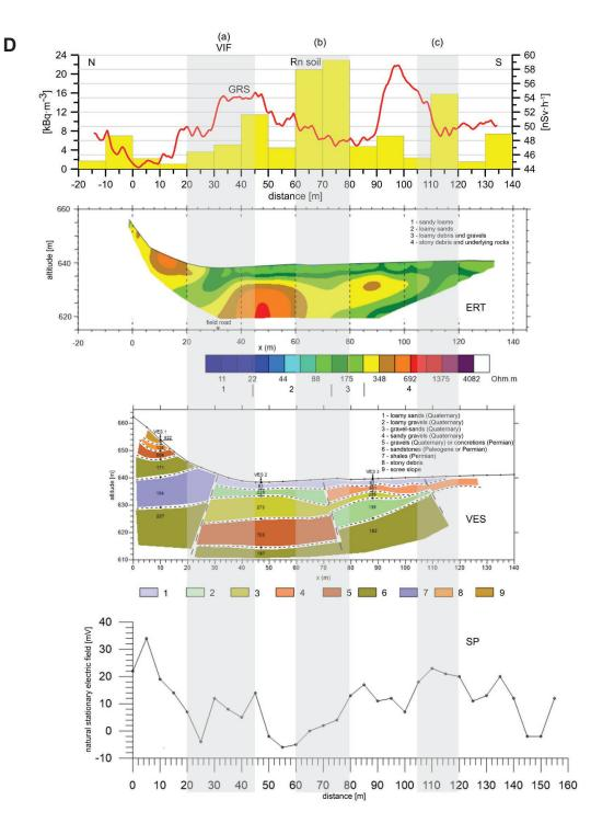
Fig. 5. (continued) Comparison of CSAMT related fault structures and shallow depth geophysical, emanometric and dowsing data. A — Kravany profile; B — Spišský Štiavnik profile; C — Vydrník profile; D, E — Spišské Bystré profiles; F — Hranovnica–Dubina profile. Geophysically detected single faults are distinguished by alphabet indications (a – VIFs.s., b, c, ...) commented in the text. Grey transparent belts mark and connect multi-method indications of the same fault-discontinuity.
