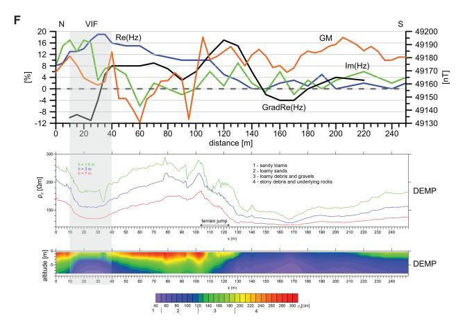
Fig. 5. (continued) Comparison of CSAMT related fault structures and shallow depth geophysical, emanometric and dowsing data. A — Kravany profile; B — Spišský Štiavnik profile; C — Vydrník profile; D, E — Spišské Bystré profiles; F — Hranovnica–Dubina profile. Geophysically detected single faults are distinguished by alphabet indications (a – VIFs.s., b, c, ...) commented in the text. Grey transparent belts mark and connect multi-method indications of the same fault-discontinuity.
