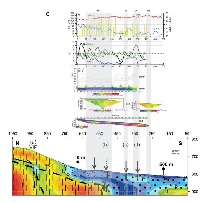
Fig. 5. (continued) Comparison of CSAMT related fault structures and shallow depth geophysical, emanometric and dowsing data. A — Kravany profile; B — Spišský Štiavnik profile; C — Vydrník profile; D, E — Spišské Bystré profiles; F — Hranovnica–Dubina profile. Geophysically detected single faults are distinguished by alphabet indications (a – VIFs.s., b, c, ...) commented in the text. Grey transparent belts mark and connect multi-method indications of the same fault-discontinuity.
